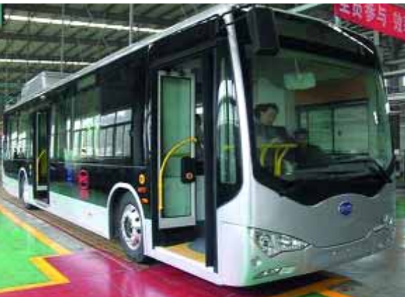
The use of an aluminium chassis and fastener components has reduced the weight of the BYD prototypes electric bus, recently launched in Changsha City, China, by a spectacular 1.2 tons
