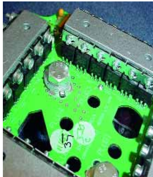
Fig 3: Control panel using HTFS which allowed for the removal of nuts and spring washers at the top of the picture
