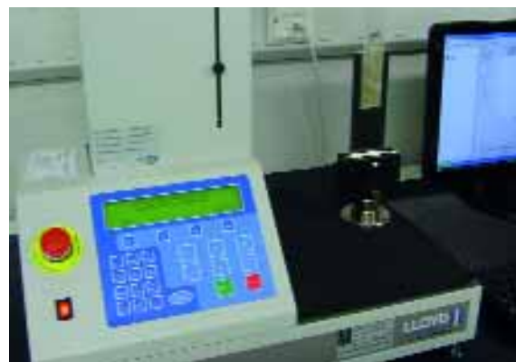
The assessment room can test materials in shear and peel
