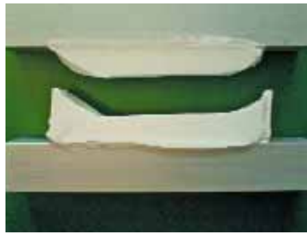
This one-component adhesive offers outstanding flexibility before eventual failure
