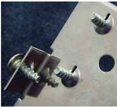
Fig 4: Example of material gauge rationalisation. Pictured above with inserts and below with the helix thread form
