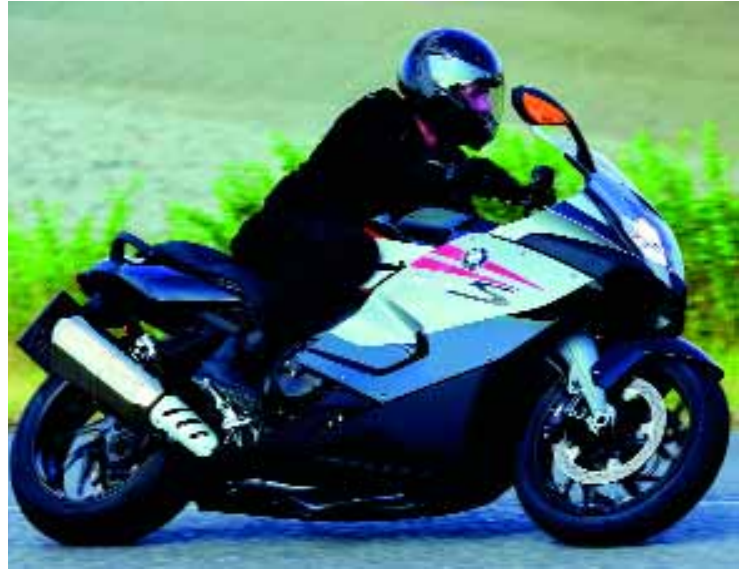
High performance BMW machines are capable of top speeds up to 140 mph by producing 175 bhp at 9,250 rpm from their 1293cc engines
