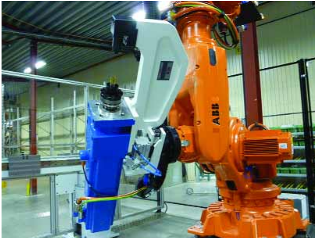
Spot-welding equipment was replaced with a modern robot cell
